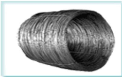
For the improvement of mechanical properties of rod wire metal the special vanadium alloy was used that allow us to reduce of vanadium content in steel on 20-40% (in relation to usual target value) at saving of necessary tensile strength 1200-1235 N/mm<sup>2</sup> depending of diameter (11-8 mm).
